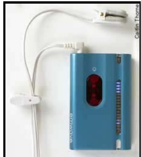
The emWave monitors a user's pulse through a clamp that attaches to your earlobe (above). It then encourages you to calm down by breathing in sync with its lights.
